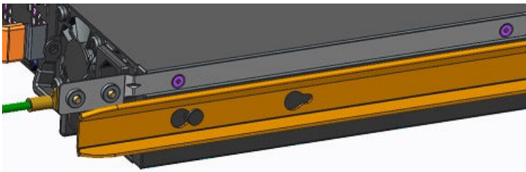
Figure 19. GND Lug/Bracket Assembly Attached to the System
